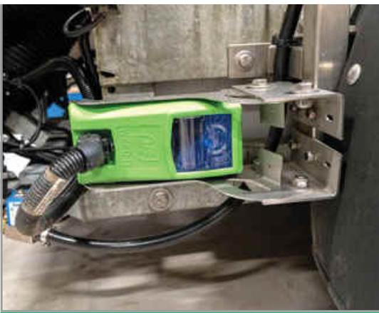
The H.S.S. I.S.A. sensor shines a light beam on the tree and measures the reflected light. The amount of reflected light is related to the foliar mass.
