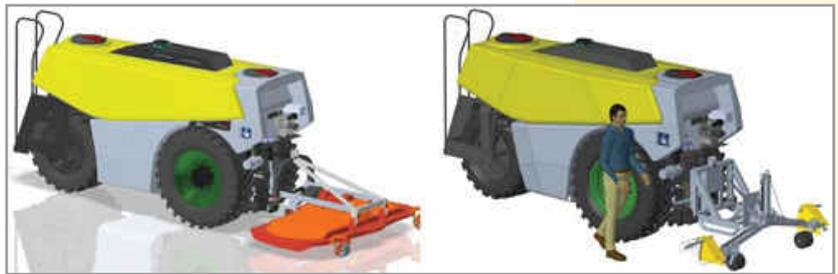
When working with a rotary mower and a weed sprayer the AgBot 3x2 drives backwards.
