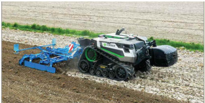
The AgBot, here with a seed bed combination, has the highest possible safety level by means of sensors and a certified GPS system.
